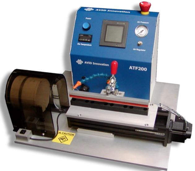
AVID Innovation's ATF200 Tip Former is the automated solution of choice for all your catheter and tubing tip forming needs. Whether your catheter tip needs a flare, taper or bond the ATF200 can be fitted with an appropriate custom die to accomplish the job.
